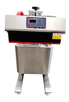
Induction sealing machine is the process of bonding thermoplastic materials by induction heating. This involves controlled heating an electrically conducting object (usually aluminum foil) by electromagnetic induction, through heat generated in the object by eddy currents.
