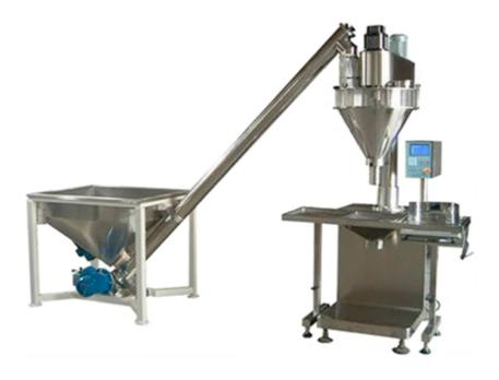
This machine is suitable for measuring and filling powder products, such as flour, milk powder, starch, coffee powder, pepper, curry powder, protein powder, spices, Chinese medicine powder, etc.
