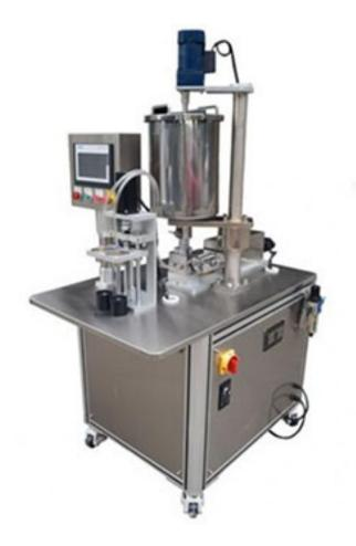
The machine is specially designed for fluid liquid CC cream filling. It is specially designed for filling air cushion BB/CC cream products, easy to operate and clean. The main part of the machine is made of stainless steel, which is easy to clean and corrosion resistant. The main electrical uses Siemens, Schneider, Omron; The gas path uses Airtac. The mechanism is compact structure, small occupation, and high efficiency, stable and reliable.
