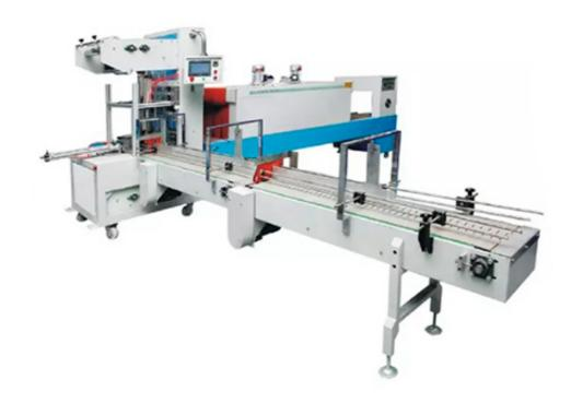
ST-6030 series sleeve wrapping shrinking machine applicable to those products need counting and lining and auto shrinking such as easy-open tin can, glass bottle, beer, mineral water etc. It includes automatic packing machine and shrink tunnel. Film Packing Machine is equipped with transducer, which can adjust various speeds for packing bottle water. It can save cost and assure the packing quality. The cutting system abides by international rules and with best sealing quality.
