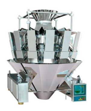
The ZM 14D25 Multi-Head Combination Weigher is a sophisticated weighing system equipped with multiple weighing heads working to accurately measure and dispense products. Developed with state-of-the-art technology, this machine is capable of handling a wide range of products, including dry goods, snacks, confectionery, frozen foods, and more. The working principle of the ZM 14D25 Multi-Head Combination Weigher revolves around precision and efficiency.
