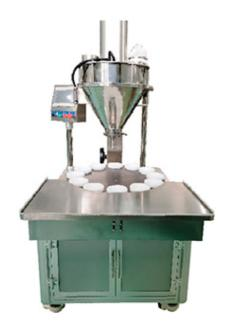
Target Products: filling machine for loose powder
