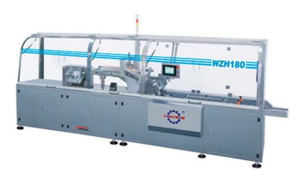
Automatic folding (1-4 folding) and conveying of manual leaflet automatic material categorizing and feeding; automatic paper carton spreading; automatic manual leaflet and material carton packaging, synchronous (3-row) batch number printing, automatic paper carton sealing, automatic waster eliminating. Al/Pl blister packs medicine plate, injection salver, bottles, ointment and rectangular or troche.
