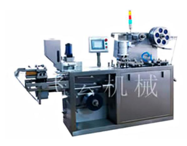
Flat plate aluminum-plastic blister packing machine is a very common machinery used in food and drug industries. Plate-type heating apparatus can heat and soften molded film and then softened molded film can be blowing molded into a blister by compressed air in plate-type molding apparatus. Product is filled into the blister in filling apparatus and delivered to the plate-type sealing for sealing operation.
