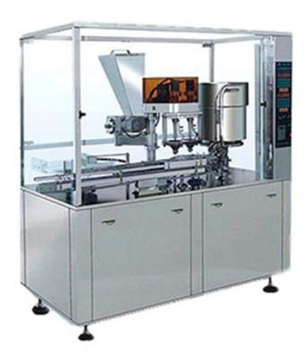
KFG2-A type powder filling machine is one kind of sterile powder filling machine which our company developed initially. Its volume is small, same direction in bottle inlet and bottle outlet. The filling and stoppering is conducted in the same graduator. With its compact structure, it is welcomed by customers with small production capacity and small room size. We have large number of customers home and abroad using this kind of powder filling machine.
