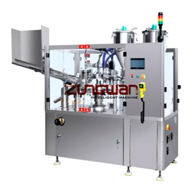
ZHF-100YD Automatic Filling and sealing Machine is mechatronic mechanical-electrical integration, use multiple introduction technology and controlled by PLC, it can complete tube feeding, local color code, filling, sealing and tube out automatically simultaneously. The machine runs smoothly, easy to control and size change over, suitable for producing paste products
