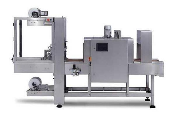
SYM-10 Automatic Heating Contractive Packing Machine - thermal shrinking packaging machine. This machine is mainly used for food, daily use chemicals, medicine and other light industrial products. Taking advantage of the shrinkage properties of shrinkable film, after the packaged goods are wrapped, they are fused with the film and then tight packaging is realized through oven. In this case, it is convenient to start sleeve packaging.
