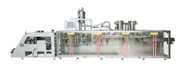
BHD-280DSC is specially designed for standard nozzle stand-up pouches, and has an additional set of workstations, which can be packaged at the same time and produce two bags, doubling the production capacity. The maximum packaging capacity is 500ml. It can be used to package soy milk, fruit juice, tomato juice, and Hanging holes, special shapes and other functions can be added according to customer needs.
