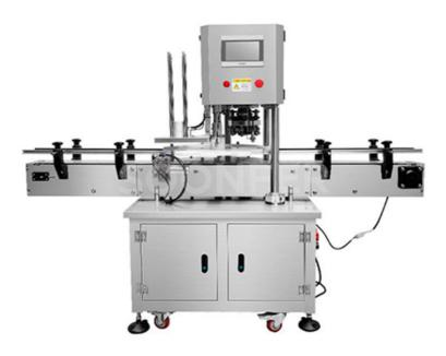
The automatic servo can sealing machine is suitable for packaging various round-mouth tinplate cans, aluminum cans, plastic cans and paper cans. Servo control makes the equipment operation more stable, safe and intelligent, and the adjustment and maintenance are simpler and more convenient.
