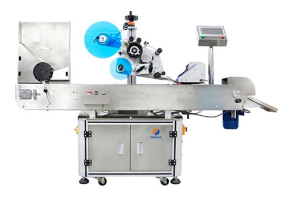
FK807 is suitable for labeling various small-sized cylindrical and conical products, such as cosmetic round bottles, small medicine bottles, plastic bottles, PET round bottles 502 glue bottle labeling, oral liquid bottle labeling, pen holder labeling, lipstick labeling, and other small round bottles etc. It is widely used in round bottle labeling in food, cosmetics, wine making, medicine, beverage, chemical industry and other industries, and can realize full product coverage labeling.
