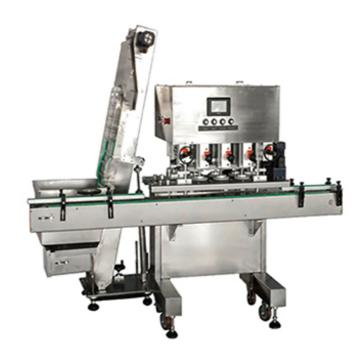
This Automatic Capping Machine is economical, and easy to operate. This versatile in-line capper handles a wide range of containers at speed up to 120 bottles per minute and offers a quick and easy changeover that maximizes production flexibility. The tightening discs are gentle which will not damage caps but with an excellent capping performance.
