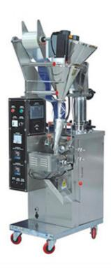
The machine is designed and manufactured specially for powdery and super fine powdery products Driven by servomotor, the auger is rotating to fill products; furthermore, the filling range can be adjusted automatically through computer. The processes of bag making, measuring, filling, sealing, cutting, counting and hot pressing codes can be done automatically. Packing material include several kinds of heat-seal lamination, such as PET/plated AL/PE, PET/PE, NYLON etc.
