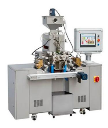
Soft capsule filling machine, fully self-service filling machine, automated filling operation
