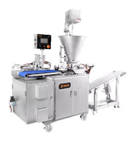
Explore the capabilities of ANKO's Commercial Empanada Making Machine! Paired with an Empanada Dough Press Machine, it requires only two simple steps to complete empanada dough pressing and forming, producing 3-6inch empanadas. We offer custom empanada pastry stamps to distinguish different flavors and for branding purposes. The production consistency and capacity ensure ideal quality products for food trucks, central kitchens, chain restaurants, and food factories.
