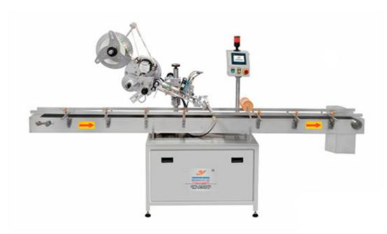
The Automatic Horizontal (Top-Side) Sticker Labeling System consists of a main structure, product transmission belt with guide adjustment, label dispensing unit, label pasting by nylon brush & sponge roller, motors, sensors, electrical panel, PLC & HMI (Feather touch Keypad), a batch printing unit (OPTIONAL), AC drives & mains ON/OFF.
