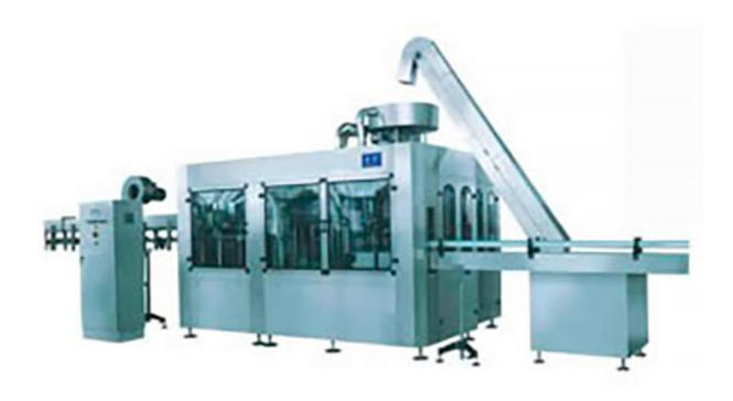
The SD-XGF series water filling machine (drinking production line) is a kind of 3-in-1 unit packaging machine. This line is mainly used for production of mineral water or pure water, as well as tea and other liquid. It is a kind of normal temperature production line that fills water in normal atmospheric temperature between 15 and 25, and it is a slew (rotate) filling machine that is popular in the market.
