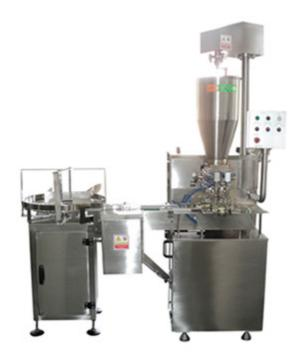
PK CFM Empty Containers are fed manually or automatically through turn table. The empty containers are carried by the belt conveyor up to the filling station. At the filling station containers are pushed forward though a chute on a platform below the filling nozzles and the filling operation takes place. After containers are filled and further pushed forward on the collection platform and the process goes on with an accuracy of +/- 0.1%
