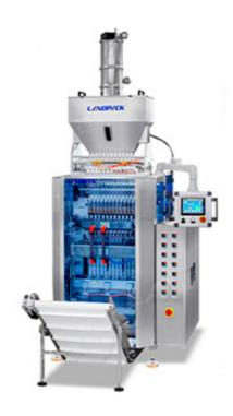
This multi lanes machine can make bags, measure, fill, seal, and make easy tearing notches. Suitable for food, cosmetics, and medicine packing such as silica desiccant, sugar, salt, pepper, washing powder, and all kinds of granules, etc.
