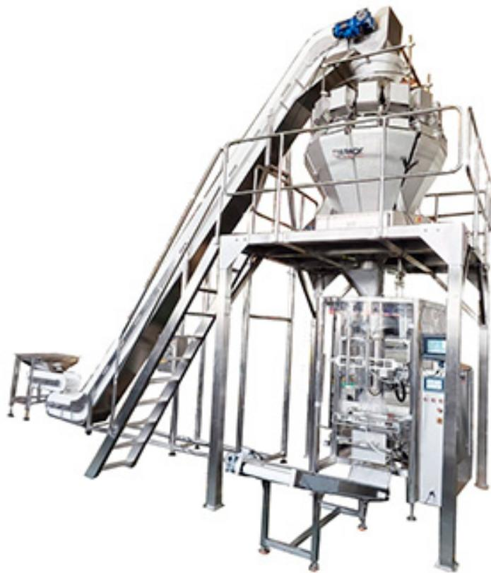
This unit machine is special design for packaging various vegetable like White radish, cucumber, lettuce, cabbage in to plastic bag. The whole machine have the function of automatic product feeding, weighing, film bag forming, bag sealing, Including date coding, bag counting. The finished bag is output from conveyor machine which no need manual collect the bag and avoid the bag polluting.
