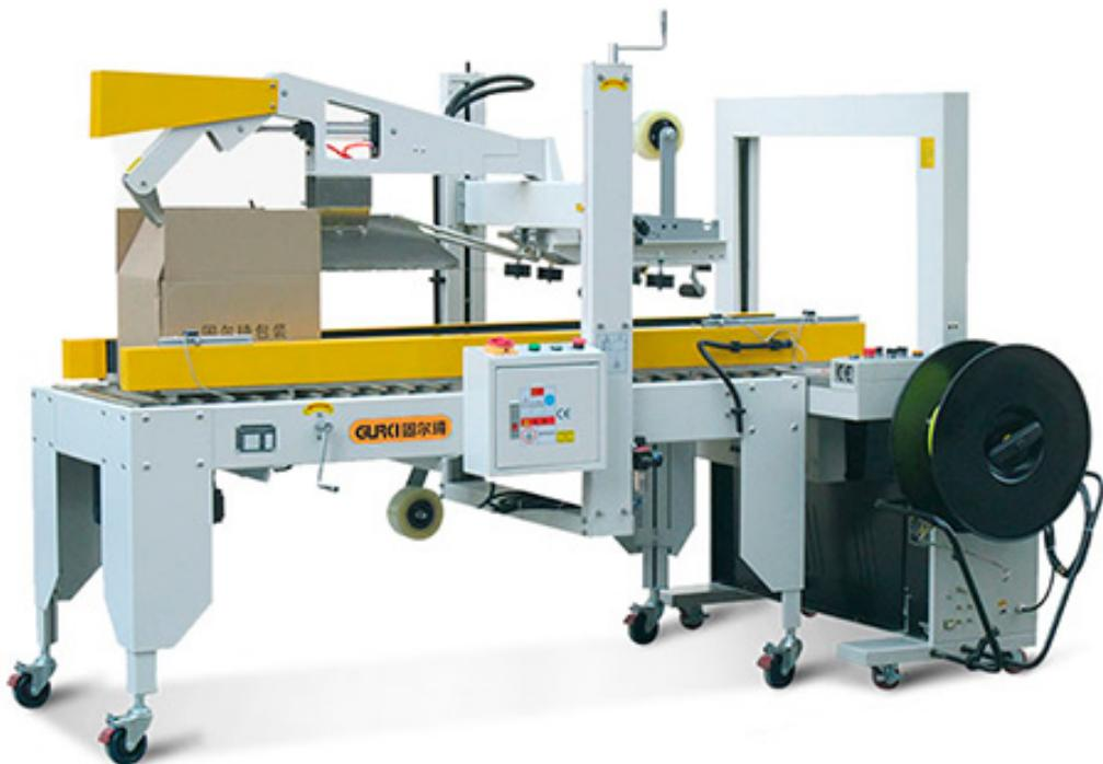
The automatic folding and strapping machine GPP-50C is a kind of packaging machine that integrates automatic sealing and bundling, and can be used with automatic packaging line. It realize automatic folding cover, upper and lower sealing tape, multi-bundling. This machine works efficiently, and can meet the needs of new and old customers.
