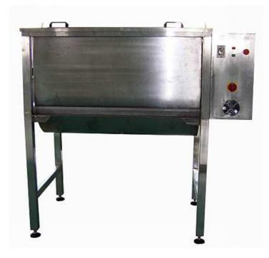
The horizontal screw belt mixer is a new type, high efficiency mixing equipment, are widely used in food and chemical industry.
