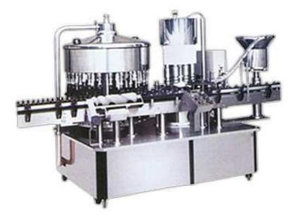
The SD-HFX-6000 rotary filling sealing machine is a kind of automatic packing machine with capscrewing ability. It is suitable for the large production of nutrition liquid, syrup, tincture and medicine for bone.
