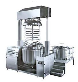
The machine is used to produce the cream the cream products in the cosmetic factory and medicine factory and especially used to emulsification of peptic material with high content of solids.
