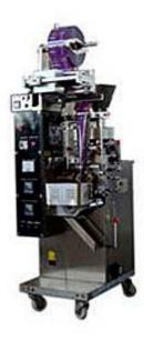
The DXDK-40II/150II automatic granular packing machine is suitable for packing non sticky, bulk or granular material, such as medical pills, food Stuffs, plant seeds, washing powder, coffee, sugar, desiccant etc The integrated processes of bag making, measuring filling, sealing cutting, counting and hot pressing codes can be done automatically. Packing materials include several kinds of heat seal lamination, such as PET/plated AL/PE, PET/PE, PAPER/PE, NYLON etc.
