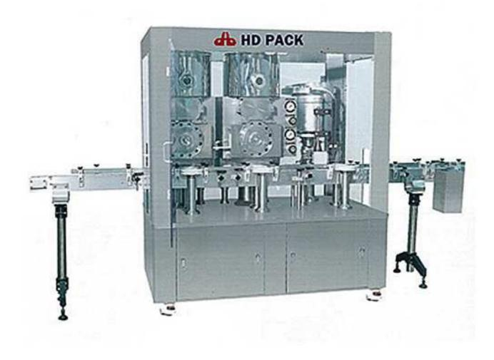
HDPVF Series, Automatic Micro Dosing powder filling machine doses antibiotic powders into vials and completes with rubber stopper. It is a vacuum type, ensuring small volume dosing between 0.2g to 5.0g precisely. All machine parts are adjustable in height to cover different sizes of vials.
