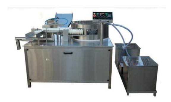
The Automatic High Speed Rotary External Ampoule Washing Machine Is Designed To Wash External Surface Of Ampoule, With 4 Stage Of Washing Which Include Washing Medium Like Detergent Water, Tap Water, Air Wash & Heating. The Speed Of The Machine Is Up To 250 Ampoule Per Minute And Can Be Varied Through Provided Speed Variation Port On Operating Panel.
