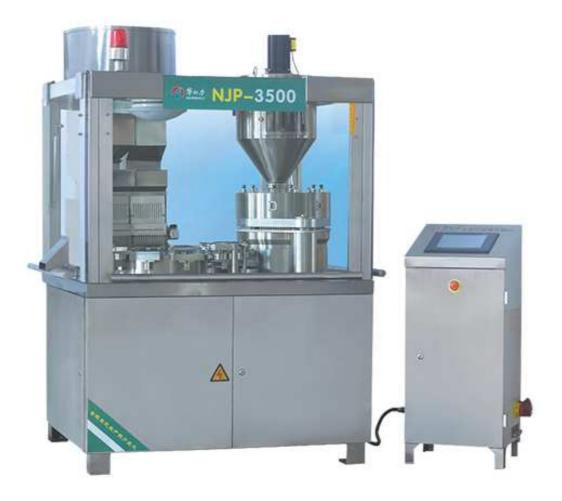
This machine is fully automatic capsule filling machines. It can produce maximum 3500 pcs capsules per minute. It is suitable for capsule size from 00# to 4#.
