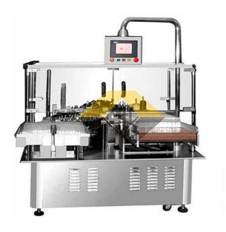
Conveying bottle system uses Discal Guide Conveying System. Conveying bottle is steady and exact. Back section, automatic pushing bottle system, is convenient for collecting, tidying and packing finished product.
