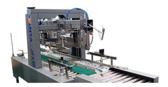
Carton Sealer is a piece of packaging equipment which automatically folds the folders of full cartons and seals them. Carton Sealers, consists of hot-melt glue carton sealer and tape carton sealer, and is suitable for beer, beverage, food and other production lines.
