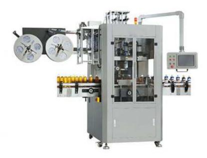
This machine adopts international technology to insert and sealing the shrink label on round, square, oblate bottle caps and body. The machine adopts high quality stainless steel and aluminum alloys abundantly to rationalize the structure and handle easily.
