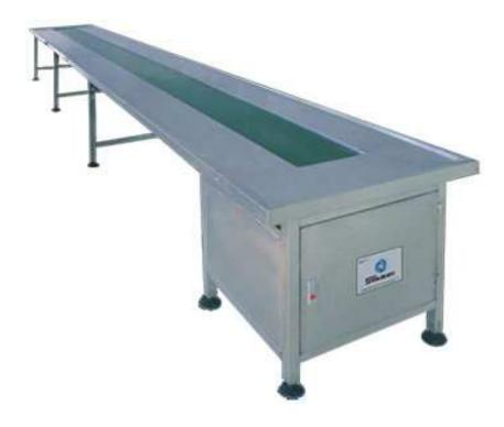
The conveying equipment produced by our company mainly includes belt type and chain scraper type with various structural forms, length 3-30 m, width and height the conveying equipment for various industries can also be customized according to customer requirements. The products have been widely used in assembly, packing production line, food, medicine, beverage and other industries requiring no pollution.
