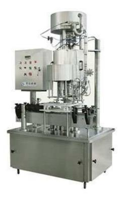
This machine is suitable for capping Glass and Plastic bottles with Plastic Screw Caps. It Easy Operation, Low Noise, Compact Design and Easy to Maintain machine is especially design for Small and Medium size factory operation. The production capacity of this machine range from 6000 bottles to 15,000 bottles per hour.
