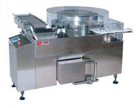
This equipment continuity type washing machine, suit to continuity produce small injection bottle (like vial bottle, ampoule, injection tub... etc) pass through ultrasonic trough oscillate, use high pressure water spray bottle interior and exterior, multiple rinsing process, Circulation water rinsing / Pure water rinsing / WFI rinsing / Clean high pressed air rinsing.
