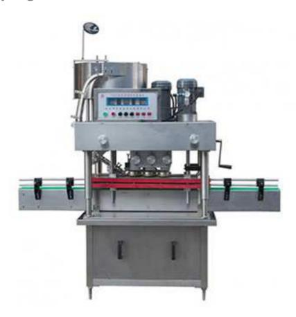
JCP-6A In-line Structure Capping Machine comes with cap sorter, cap falling rail, bottle-tightening structure and capping wheels. By tightening the belts, the bottles avoid cap scratches, push and capping thus applies to capping of round and flat bottles. This capping machine has solid structure and easy adjustment. Minor adjustment when changing bottle type, no hassling of part changing.
