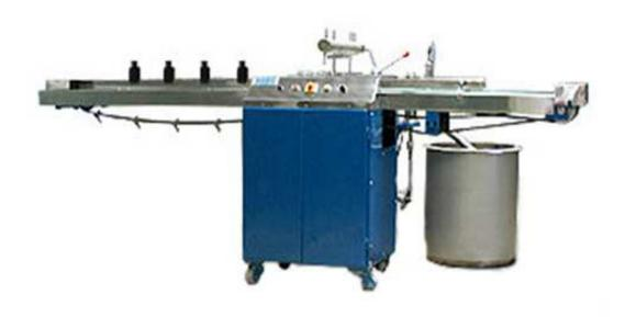
Semi-Automatic Liquid Dosing Machine with conveyor and syringe type of pump to take predetermined doses from 3ml to 200 ml in glass bottles, glass tumblers or any other packaging containers.
