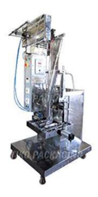
The MK-203 is a semi pneumatic vertical form fill and seal packaging (VFFS) machine designed to package various viscous and paste type products. This machine uses volumetric paste pump dosing system to produce center sealed and 3 side sealed pouches / bags.
