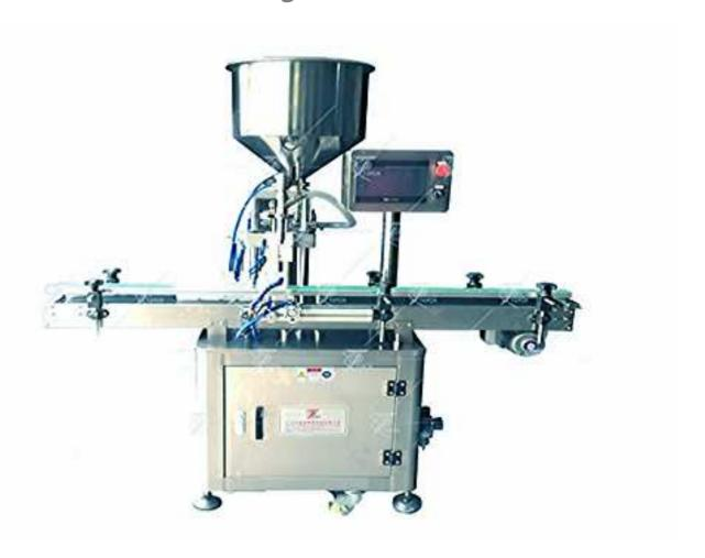
Single head Automatic plastic bottle 10-250ml pneumatic liquid cream filling machine has 1 filling nozzle. This Machine adopts serve ball-screw system to drive the piston cylinder. It's widely used in Food, Chemical, Medical, Cosmetics, Agrochemical industry, applicable for filling liquid, especially for high viscosity material and foamy liquid, such as: Oil, Sauce, Ketchup, Honey, Shampoo, Lotion Lubricant oil, etc.
