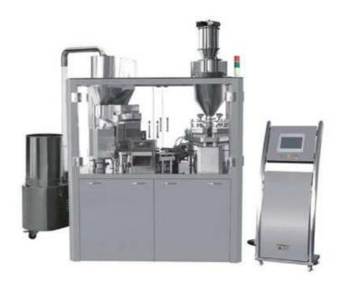
The SED-3800J Automatic Capsule Filling Machine, Automatic Capsule filler, high speed capsule filling machineprocesses the products for optimal productivity up to 3800 capsules per minute, featuring low-maintenance operation, minimal downtime, and overall dependable production. Powder dosing uses the 5 stage tamping technology for an enhanced accuracy. Filling of pellets is available.
