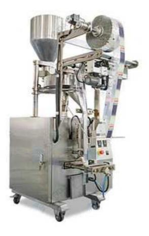
F100B-R Automatic Three Edge Small Sachet Sealing Packing Machine is specially designed for powder material auto-weighing filling and bag forming sealing. Widely applied in the market of chemical powder, food powder, additives, this machine unit has been accepted by customers for a long time.
