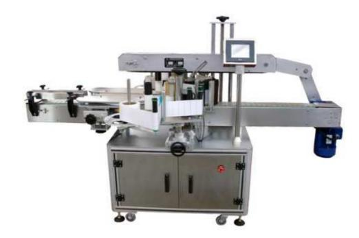
Adhesive labeling machine consists of conveyor system and label-guide system. conveyor system can be customized and adjusted according to customer's needs. Label-guide system can label right product location when sensor check products.
