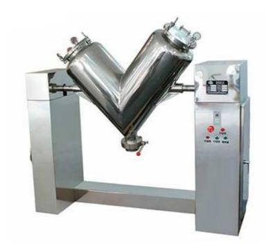
V Type Mixer is primarily used for mixing dry powder, granulate or crystal products in Chemical, Food, Pharmaceutical and other industries. By rotating the V shaped vessel, the materials move in convective motion to get a quick and homogenous blending.
