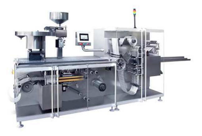
This machine is suitable for automatic high speed alu pvc packing of capsules, tablets and chewing gums, candies. It adopts flat pressure forming to form strong and average blisters. and roller type mesh sealing to ensure reliable sealing. The machine is equipped with batching system, embossing device and horizontal boundless punching to achieve high production capacity and greatly save packing material.
