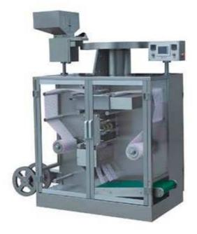
This aluminum strip packing machine is suitable for automatic double aluminum foil packing for tablets and pills in medical medicine, chemical industry, foods etc.
