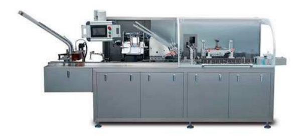
The machine adopts horizontal machine, continuous transmission, stable running, high speed, the product is suitable for use in medicine plate, bottles, hose, soap, poker and other drugs, food, cosmetics, daily chemical industry such as packaging, its performance characteristics are as follows:
