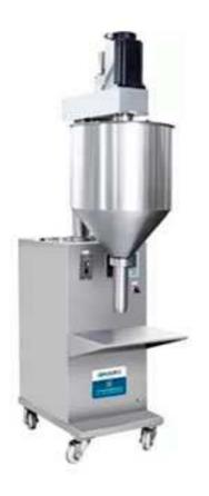
Sanitary grade semi-automatic show gel filling machine piston is suitable to fill the honey materials with high viscosity and poor flow ability. It does the filling pneumatically, its hopper and the cylinder both are thermally preserved with electrically heated circulation water. The hopper is equipment with a frame mixing system. The machine is easy to clean and operate. Confirming to GMP standard.
