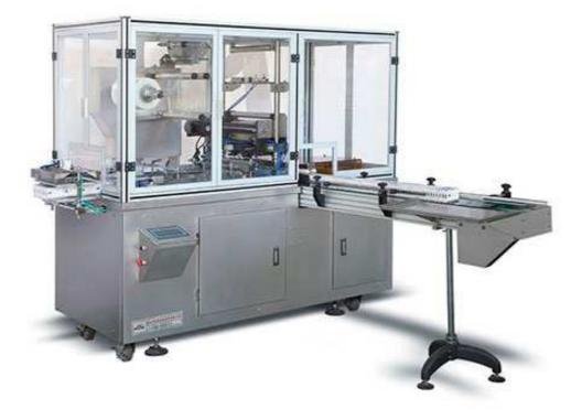
The KX-400C-1 cellophane overwrapping machine carries out feeding, stacking, wrapping, heat seal, sorting and application of anti-counterfeit tear tape. It is widely used for cellophane overwrapping of pharmaceutical, health care products, food, cosmetic, audio-video products, stationery, daily necessities and more.
